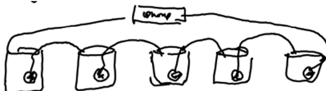
Figure 1: for 12 Volts you need at least 5 systems wired up in series
