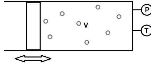
A cylinder with initial volume  $V = 2\text{ L}$  is filled with nitrogen. The cylinder is hermetically sealed by a piston. In the first part of the task, the piston is blocked, the gas is heated to different temperatures and the pressure is measured for each temperature. The results of the measurements are shown in the following table.
