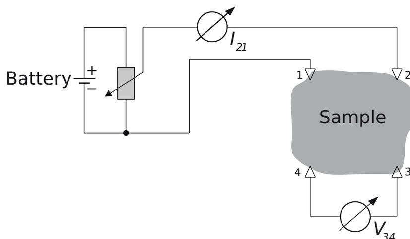
For symmetry reasons  $R_{21,34} = R_{34,21}$  and  $R_{14,23} = R_{23,14}$ . Van der Pauw showed that for an arbitrary but
