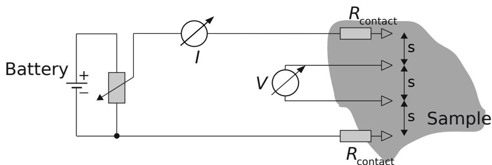
The curve  $I$  versus  $V$  represents the  $I - V$ -characteristics of the sample and allows the resistance of this sample segment to be determined. In the following we will only use the 4PP technique. To start, we will use the linear *equidistant* arrangement of four out of the eight probes (contacts) shown in the photograph.
