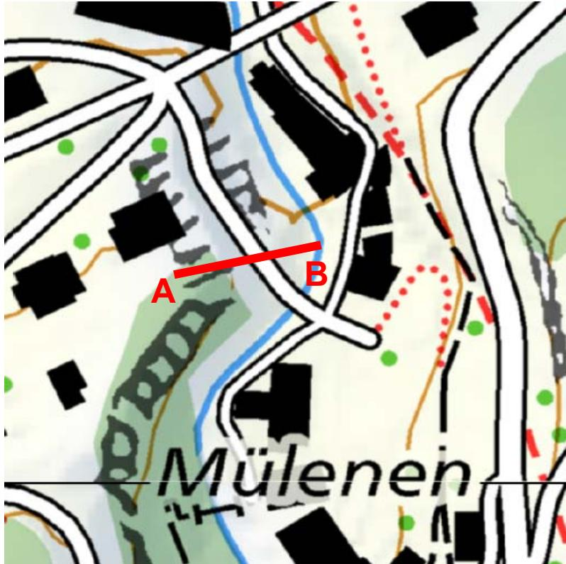
1.1) Estimate the height of the highest point of the rock face (Point A) by using the maps with the scale 1:5000 and 1:2500.
